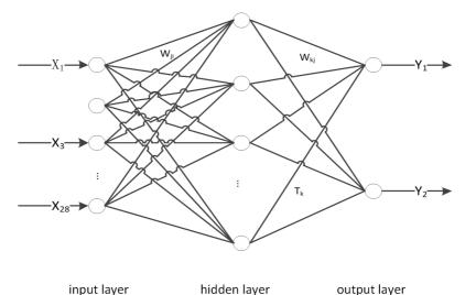
Fig. 1. Three-layer BP network structure for gait analysis
